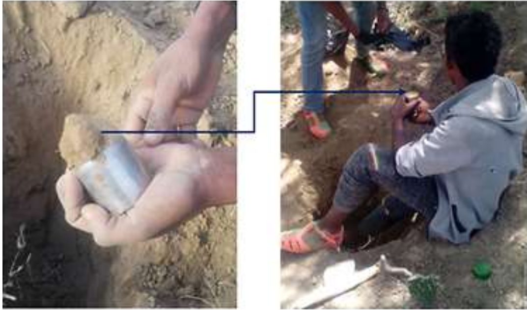
Figure 3. Remove excess soil from the bottom of cylinder with knife.
